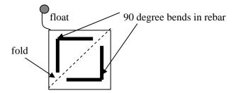
This small (5' x 5') benthic mat can fold diagonally for easier deployment and positioning by one person on uneven substrate. The rebar sections are not connected to each other at two of the corners, allowing the barrier to be folded. A float is attached at one corner to help locate the mat.
