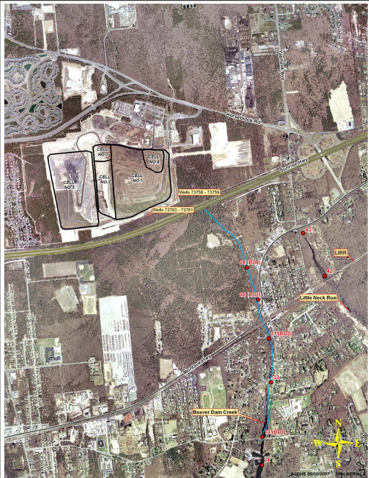
Figure 14. Brookhaven Landfill Showing Locations of Cells 1 through 5 and South Perimeter Monitoring Wells (73758, 73759, 73761 & 73763)
